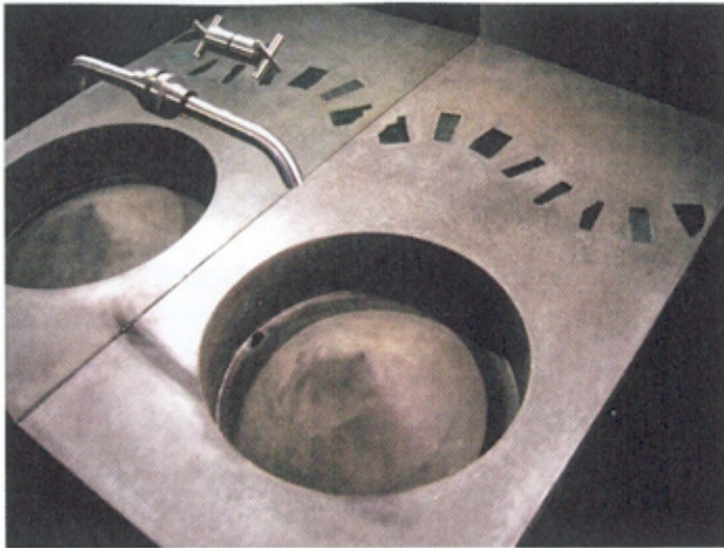
The Best Integral Sink achieves Chris Frazer's objective of creating something out of the ordinary. "The 18 in. (450 mm) cone forces water to the outside, and a 2-degree pitch at the bottom has water go around back to drain," he said
