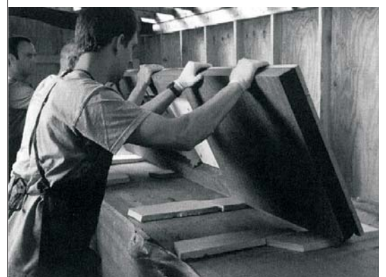
Image 4. Carefully turn the counter over
