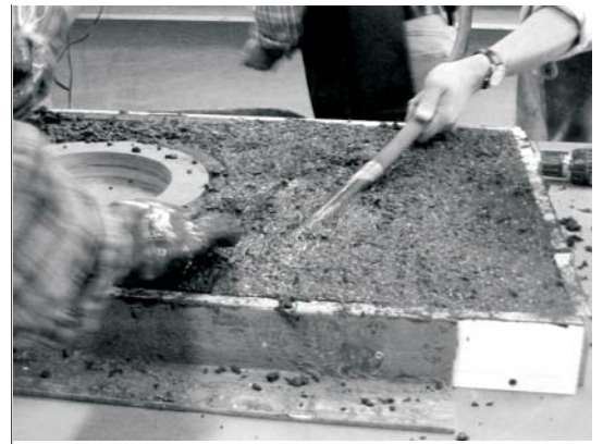
Image 2. Vibrate the mix in layers
