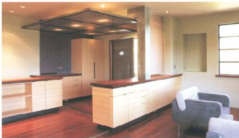
Above: The island supports a large three-inch thick mahogany prep table cantilevered over a sculptural, freestanding concrete pedestal with integral sink ■ Below: A soffit made of steel and translucent honeycomb Panelite defines the foyer ■ Bottom: The stepped charcoal-color, concrete hearth sits below an eggshell-colored plaster fireplace façade with geometric, steel-framed vents. The dining area is next to the living room area in the same room. The kitchen lies through a wide doorway
